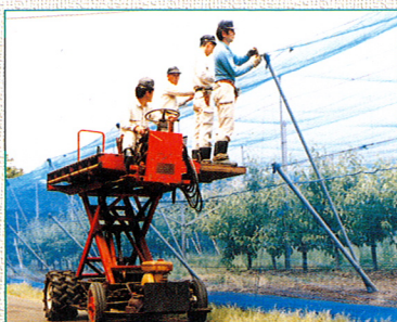
Installation of a bird protection net using a vehicle for high-place work
