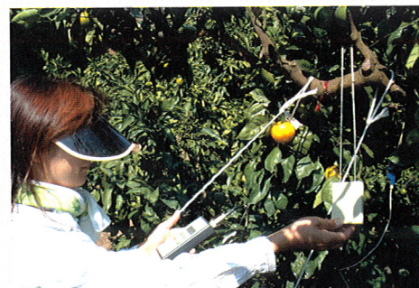
Measurement of volumetric water contents in citrus trees
